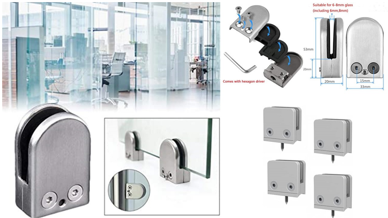
Figure 4: Examples of glass clamps to enable safety tie-down of glass plates. The thickness of glass used with these commercially available clamps are generally thicker than the devices for the experiment. The mismatch can be resolved by placing a 3mm-thick piece of plastic shim, about 1-by-1 inch or slightly larger, that both leads to good thickness fit and also distribute the point force over a larger area. The color of the plastic should be made to match that of the mirror and glass devices.
