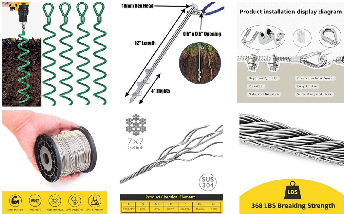
Figure 5: Examples of ground anchor and stainless steel cable for tie-down. We suggest 1/16 inch (1.5 mm outer diameter) stainless steel cables for the tie-down. a minimum gauge of 1/32 inch is necessary for the expected loads. Commercially available parts for cable handling and adjustments are also illustrated.
