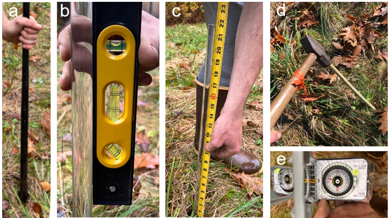
Figure 6: Techniques for perfect array geometry. (a) A metal stake is used for pre-drilling holes for planting the glass rods. Letting gravity act on the center of the gravity of the stake ensures verticality. (b) A level is essential for checking verticality both during pre-drilling with the stake and upon installation of the glass rod. The measurement needs to be performed from both orthogonal direction. (c) The implantation depths (different from that illustrated) need to be precisely controlled. The goal is to achieve 50 cm distance between the air-soil interface and the center of the plate. (d) When using a smooth, featureless rod for tie-down, the anchoring stakes need to be inserted into the soil at an angle such that it makes a angle less than 90^\circ with the tension cordage. This is to ensure that no slipping off from the tip could happen. (e) A compass that provides geographic North (instead of magnetic North) is necessary for both establishing the orientation individual devices, and for planning out perfect rectangular arrays precisely oriented parallel and orthogonal to the cardinal directions.
