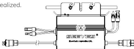
**Step 3: Connect microinverter AC cables serially**
